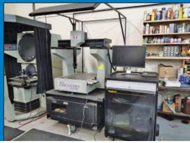
Elox Wire EDM, G&L Discovery CMM, 50" X 80" Sheffield CMM, 20" Deltronic Optical Comparator
