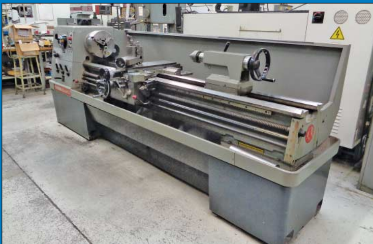
17" x 80" Clausing Model Colchester 17" Engine Lathe
