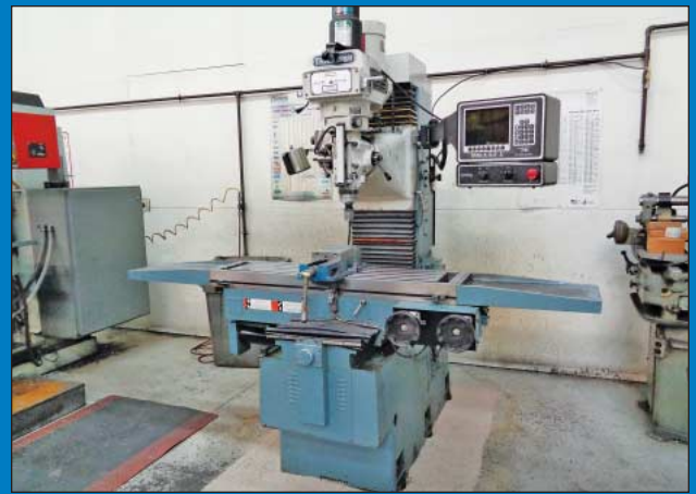
SWI Trak Model DPM-5 CNC Bed Mill
